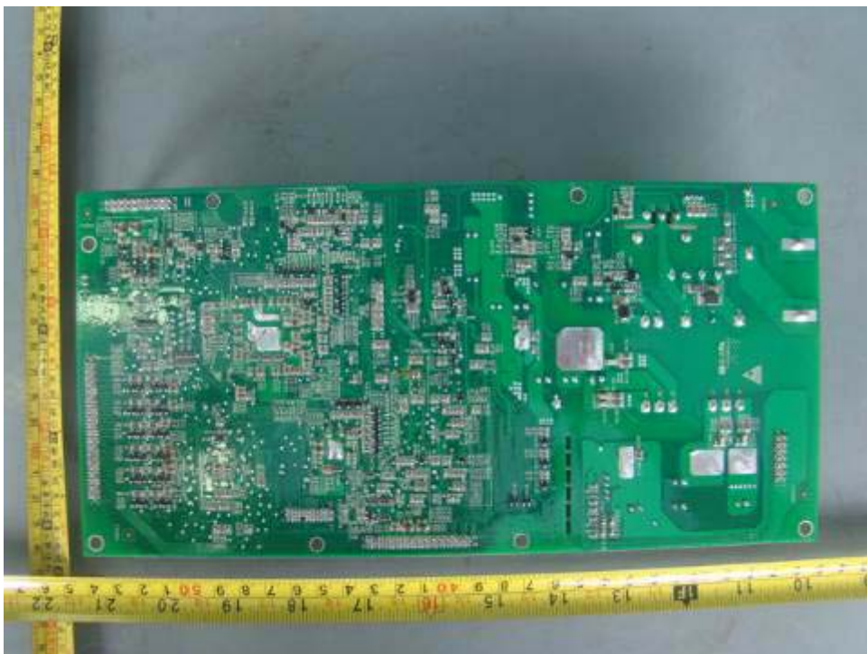
Trace side of control board
